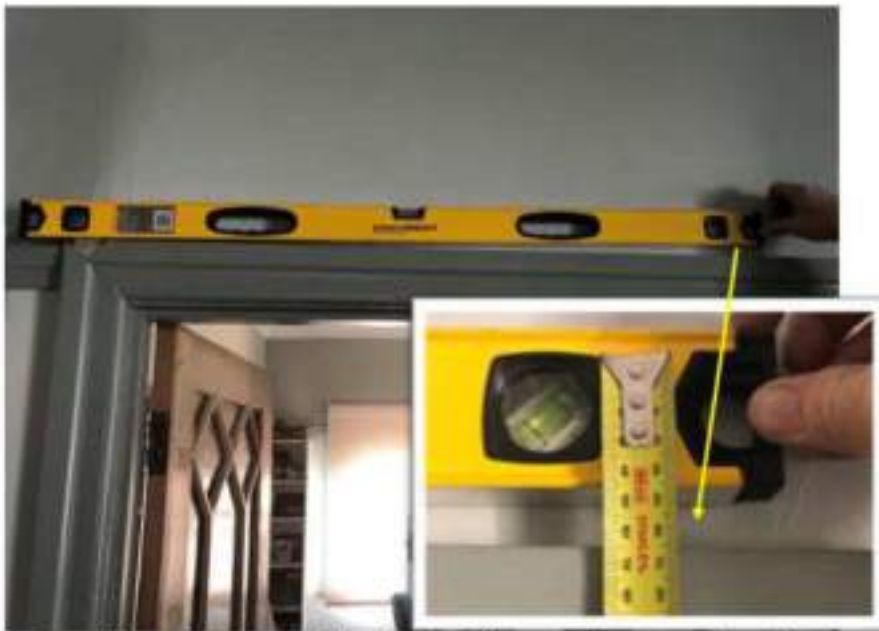
French door frame out of horizontal alignment by approximately 20mm/m
