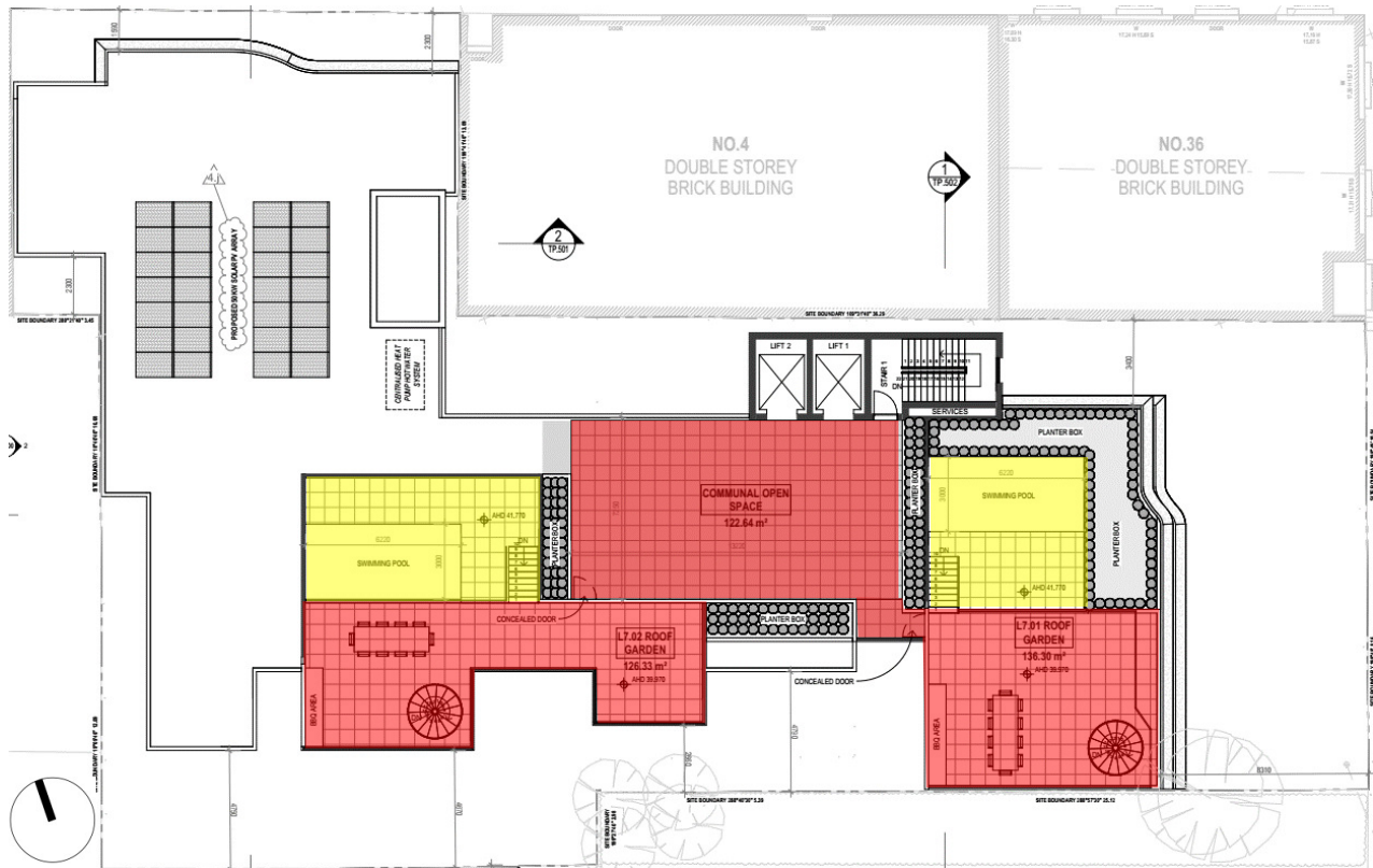
Figure 10: Roof plan with recommended wind criteria overlaid.
