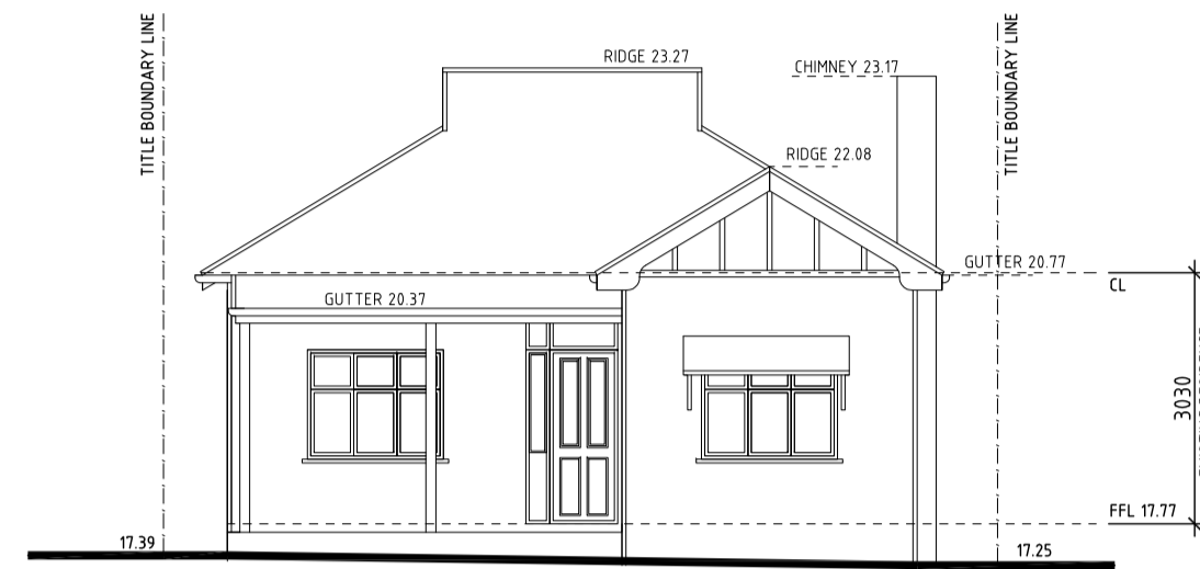
EXISTING WEST ELEVATION
