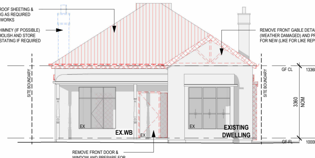
NORTH ELEVATION (EXISTING)
