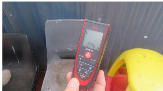
Laser measuring device used to measure the distance between the site boundary (as delineated by the existing fence) and the wall of the dwelling at 120 Creswick Street in which the above three windows are located. The measurement was just over 2.6m. Although we did not measure the width of the eaves above the windows, I estimate that they (including the gutter) would be about 0.6m wide, so that there would be a distance of 2m clear to the sky between the windows and location of the proposed toilet building. Even if they are slightly wider, there would still be more than the 1.6m dimension required by Standard B4-1
